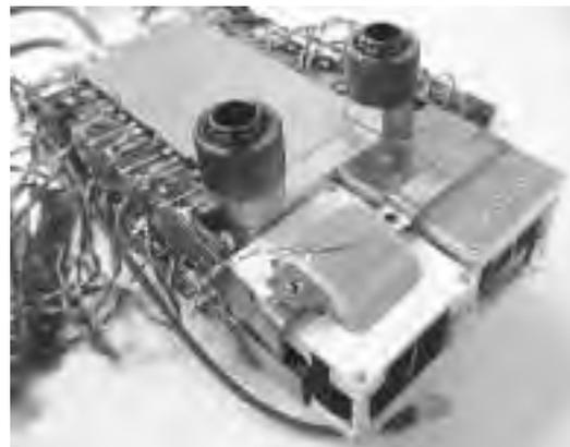
Figure 16: Integration of two converter modules into single converter structure
