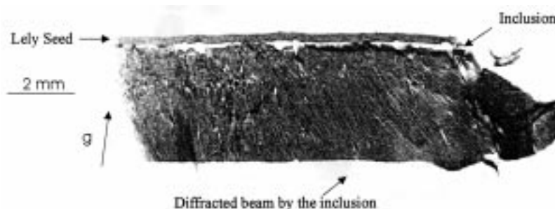
図2 6H-SiCのレーリー結晶のC面に成長させた6H-SiCの垂直断面トポグラフ写真 Fig. 2 Vertical section topography of a 6H-SiC ingot grown on the C-face of a Lely 6H-SiC crystal.
